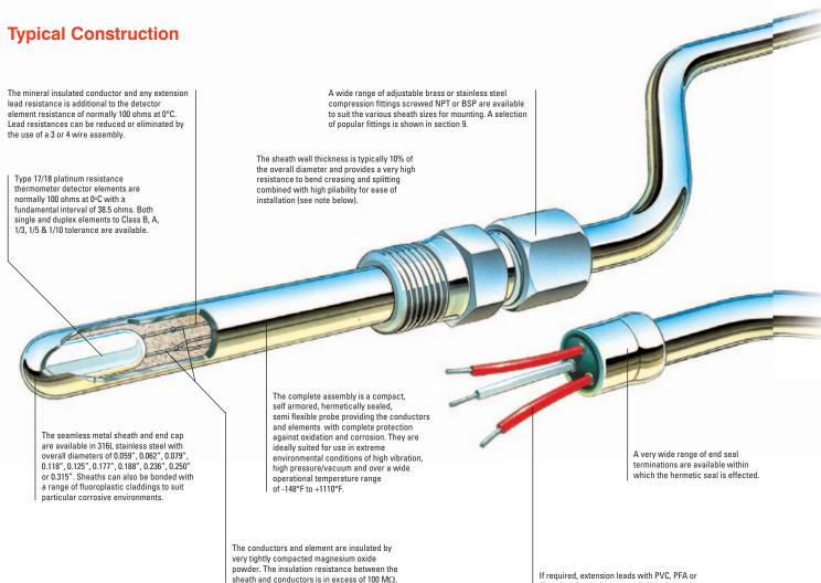
NB. The sheaths of these assemblies have a nominal bending radius of 12 times the sheath diameter. This can be reduced to 4 times the sheath diameter given the careful use of a mandrel and bending in one set. The sheath should not be bent or worked within 50mm of the tip of assembly.
